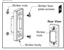
**9.** Insert the striker body, with the striker face plate screws and the striker nuts attached, into the cut out in the closing jamb.
