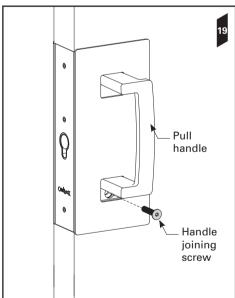
**20**. Close the door and push the *pull handle* down into the 'locked' position. Insert the second handle joining screw through the top hole and tighten.
