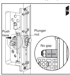
15. Place the small end of the second spanner across the flats under the head of the *plunger*. Keep the spanner restraining the plunger nut stationary while turning the second spanner clockwise. Continue to turn the spanner until there is no longer a gap between the spanner and the shroud face.
