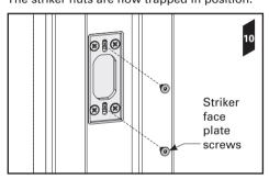
**11.** Position the striker face plate in the centre of the striker body - this may need to be adjusted in the steps following. Insert the striker face plate screws and loosely tighten.
